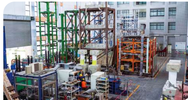
NCREE has a 5-meter by 5-meter Tri-Axial Seismic Simulator for earthquake simulations on small structures.
